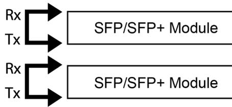
2. Each channel should auto-negotiate with itself, turning its Link Status LED on.
